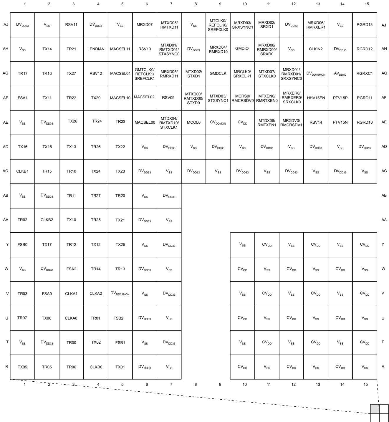
Figure 2-2. C6472 Pin Map (Bottom View) [Quadrant A]
